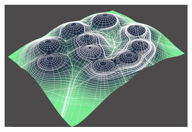
Figure 7. A NURBS surface with equipotential and stream lines texture where point charges coincide with attraction points
