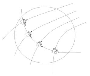
Figure 1. Vectors  $\sigma_1$  and  $\sigma_2$  at four points and the associated streamlines
