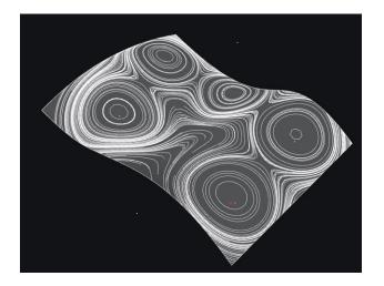
Figure 5. A generic NURBS surface with equipotential lines related to five point charges
