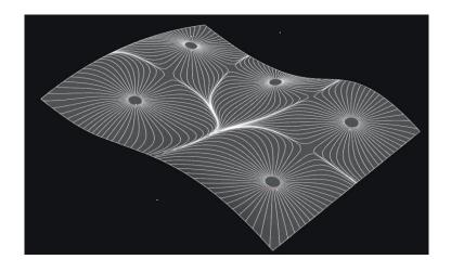
Figure 2. Force field applied on an arbitrary NURBS surface
